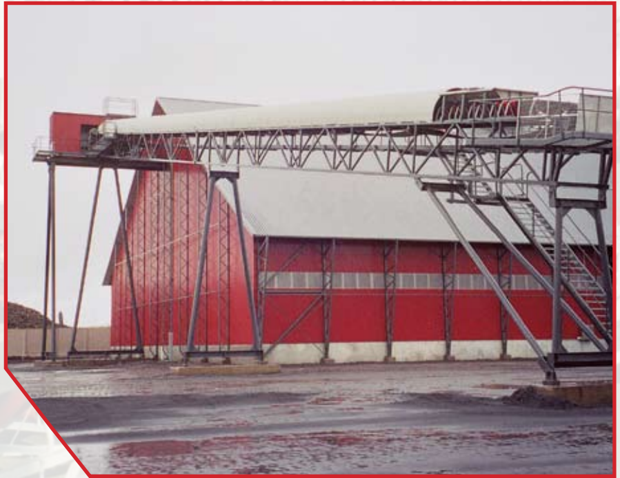
Ilmenite conveyor, capacity 1500t/h
