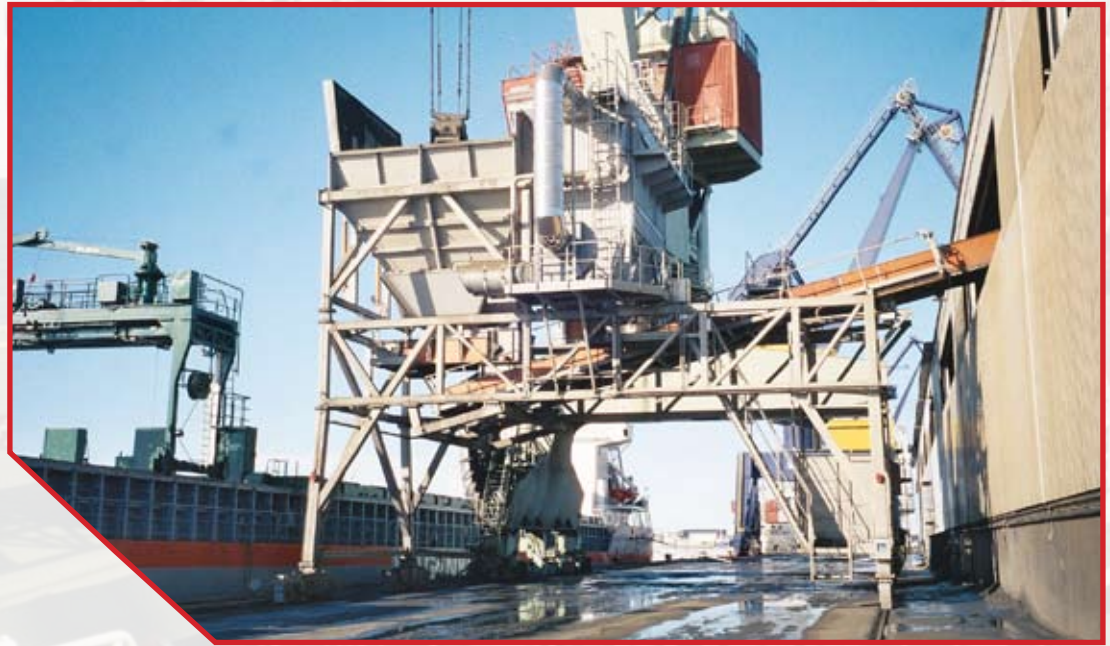
Efficient conveyors, capacity 1500t/h
