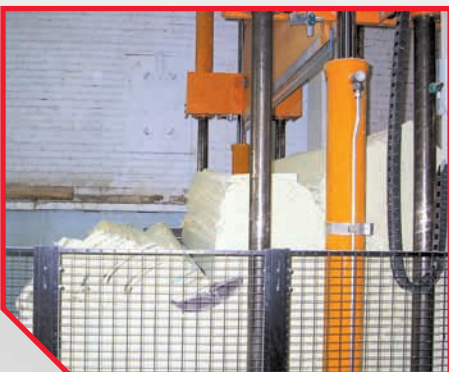
The whole working sequence is protected against unattended approach. No access to blade working area.
