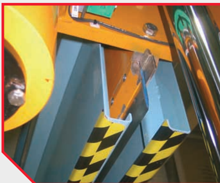
The blade is protected in its rest position.
