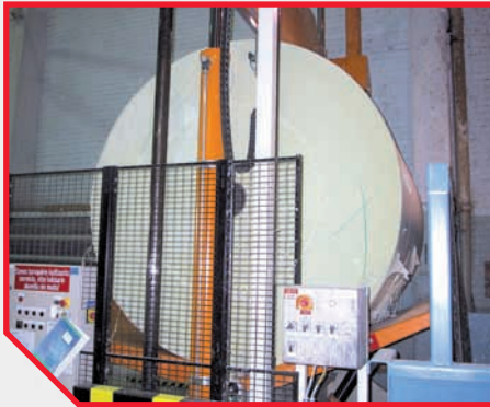
Roll adjustment to cutting position by means of covers.
